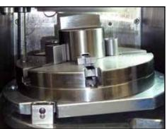
**The Premia Sharpening System includes** a graduated angle plate that allows a shear (rooftop, whisper, or one-way) to be ground on to punches easily. Simply tilt the plate and use the graduated cam to select the appropriate angle up to 12°.
